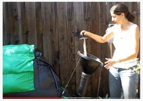
HomeBioGas is a bacteria digester that transforms organic waste such as food scraps and manure into methane gas for cooking. It also produces liquid fertilizer as a byproduct. The device needs a warm climate for bacteria growth. -GEG
